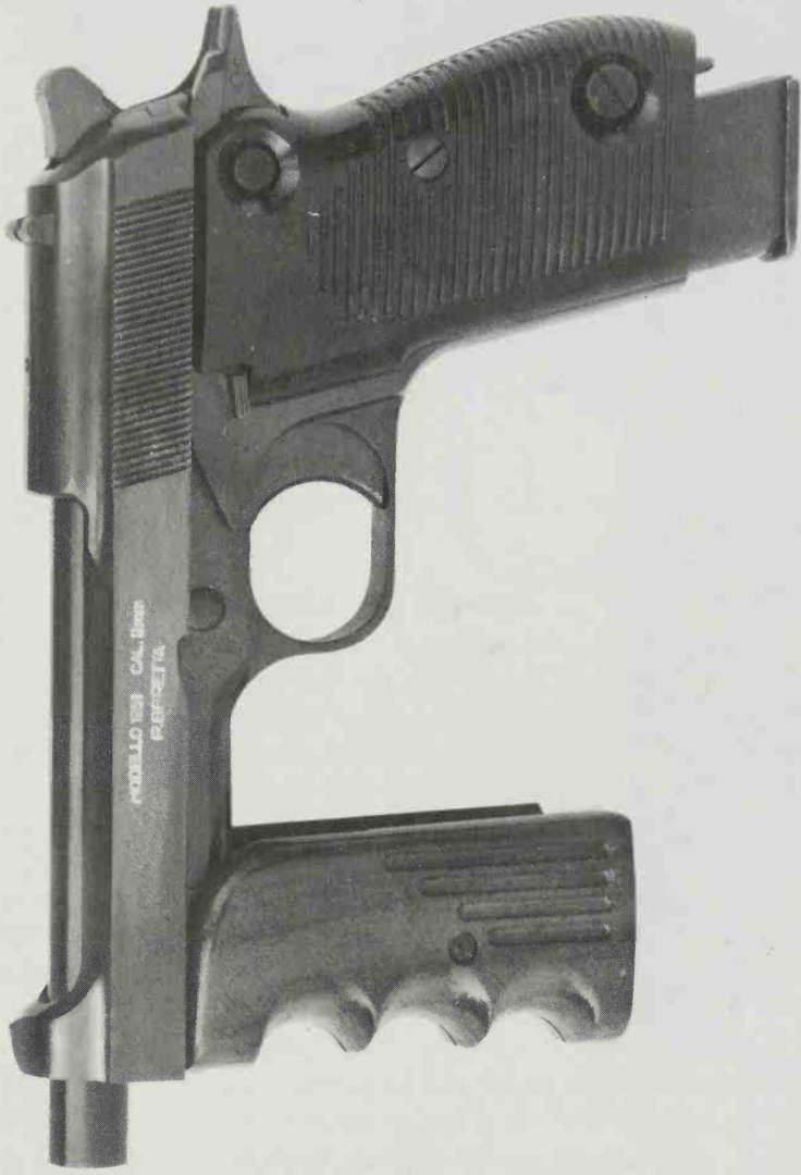
The Model 951A (951R), an experimental selective-fire pistol. The front handgrip could be folded to the rear when not in use. (Beretta Archives)
