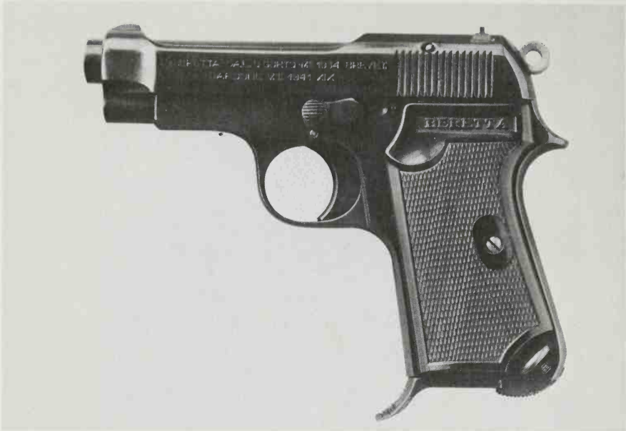
This late-style grip probably was not used as early as the date on this Model 1934 (1941) indicates. Perhaps it was an experimental version tried on an existing pistol. (Beretta Archives)
