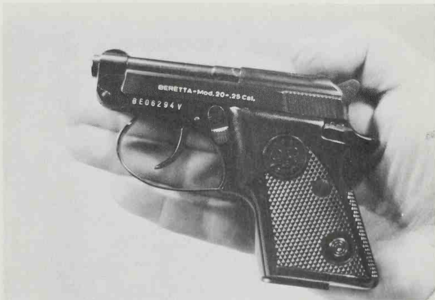
An early production U.S.-made Model 20. Note the slide marking, and the concentric ring magazine release button. (Author's Collection)
