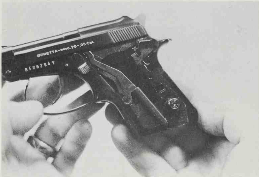
The recoil spring system of the Model 20 uses the same principle as the 950 Series pistols, but the mechanical application is entirely different.
