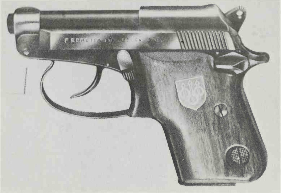
An early prototype of the Model 20 pistol. The frame apparently was converted from a standard 950 Series type. (Beretta Archives)
