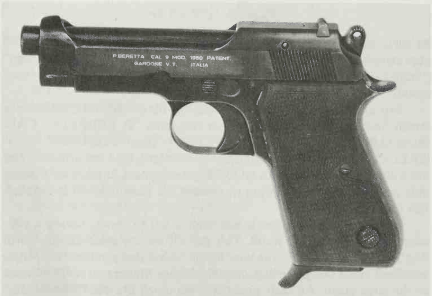
The initial post-war prototype in 9mm Parabellum. Except for the magazine catch, it is still an enlarged 1934-pattern gun. (Beretta Archives)
