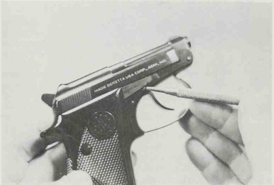
The double-action trigger uses an external drawbar, located on the right side of the frame.
