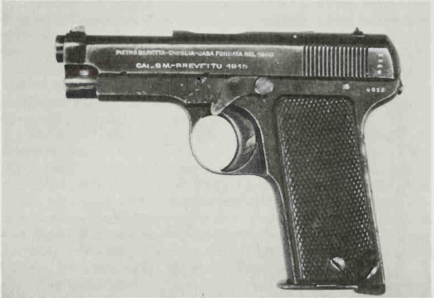
A later Model 1915 9mm pistol, serial number 4012, shown with the manual safety in off-safe position. (Author's Collection)
