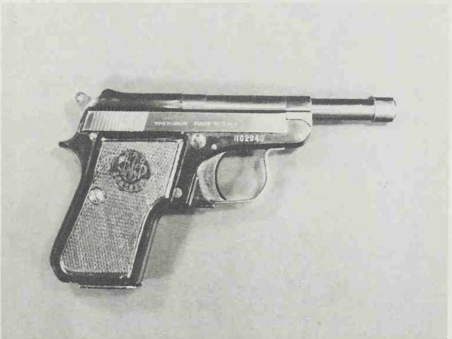
A mid-production example of the long-barreled version. Note that it is marked "Mod. 950B". "TIPO FLOBERT" is marked on the right side.
