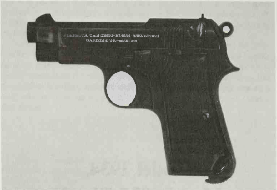
One of the specially-modified test pistols submitted to the Italian government trials, early in 1935. Note the Walther-style firing pin block safety. (Beretta Archives)
