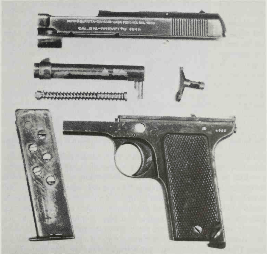
Model 1915 9mm pistol number 4012, field-stripped. Note the single mounting post at the rear of the barrel, and the captive recoil spring unit. The magazine shown, with separate counter-openings, is different from those usually found in this model.
