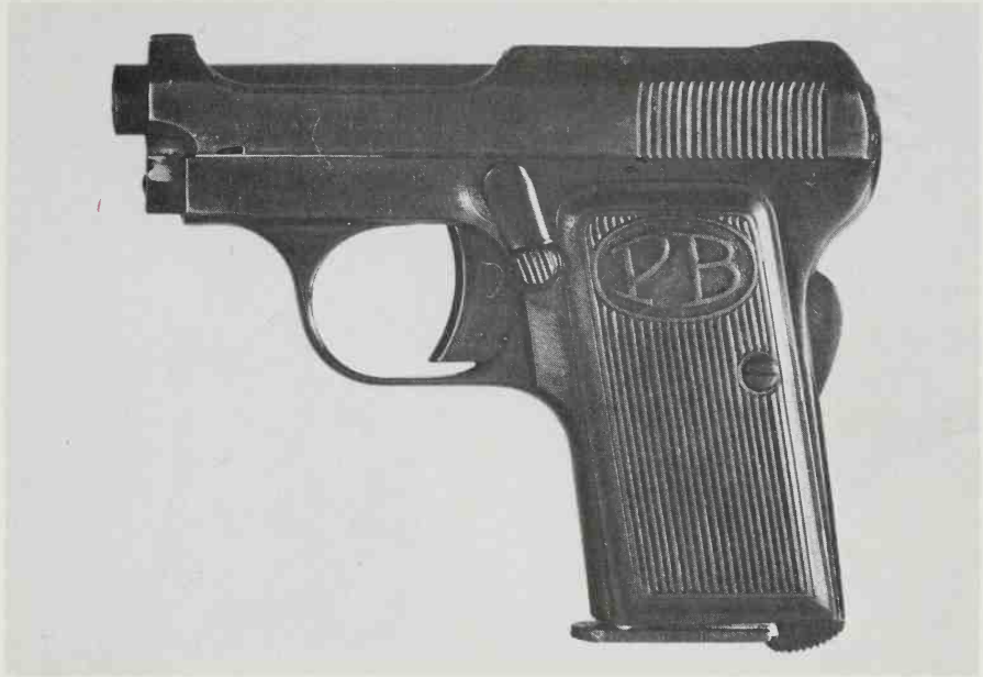
This early Model 1919 pistol has the grip safety, but was made before the addition of the disconnecter on the trigger bar. (Beretta Archives)
