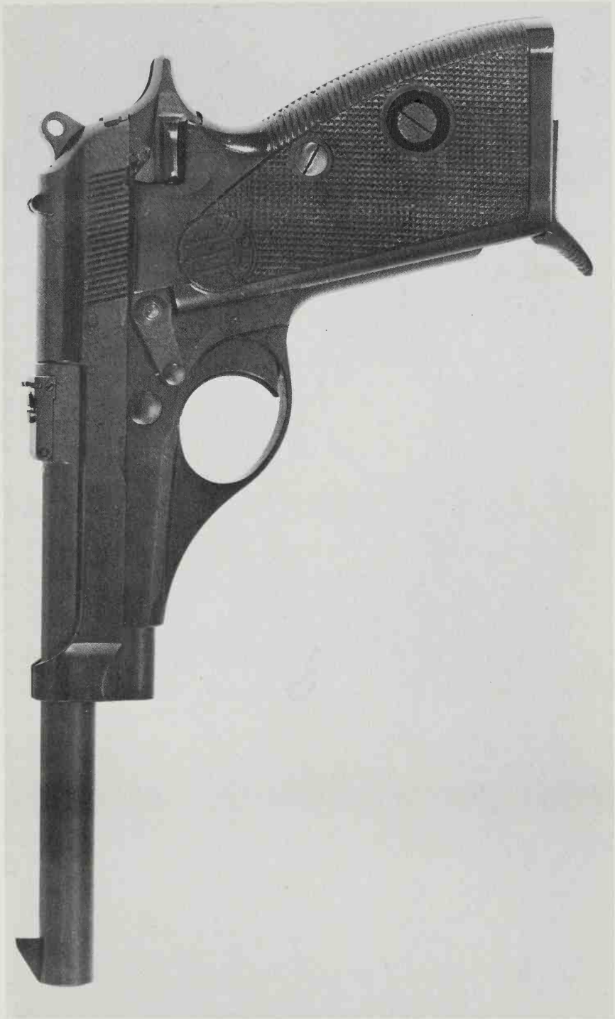
The late Model 74, essentially the same as the early version, but with a different safety and slide latch. (Beretta Archives)
