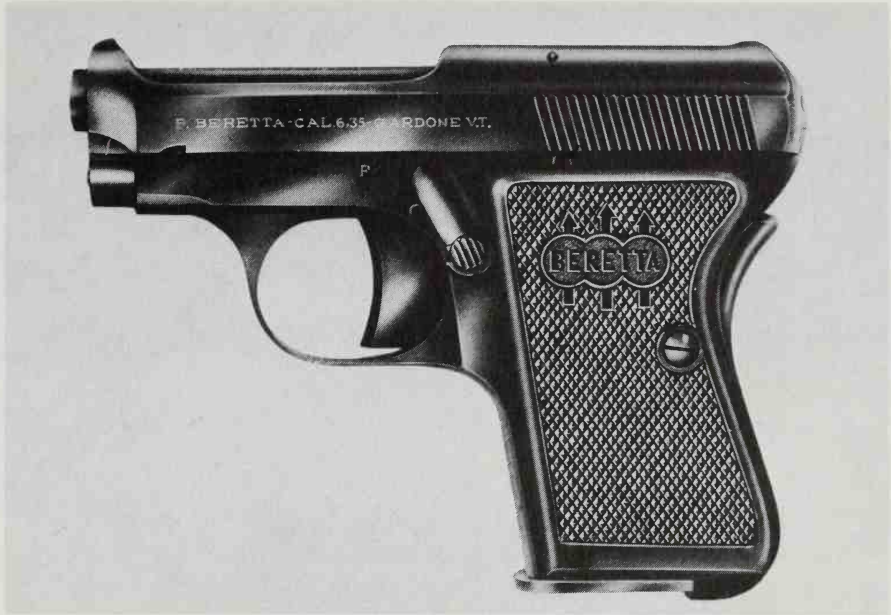
A Model 418 pistol, showing the changes of 1947. The principal changes were in the grips, magazine floorplate, and the shape of the grip safety. (Beretta Archives)
