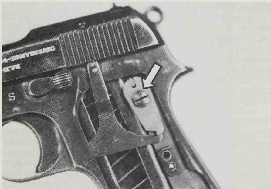
The flat sear lever of the Model 1934 is retained by a hexagon head screw (arrow) that must not be turned down tightly. Snugging the screw will bind the sear lever.
