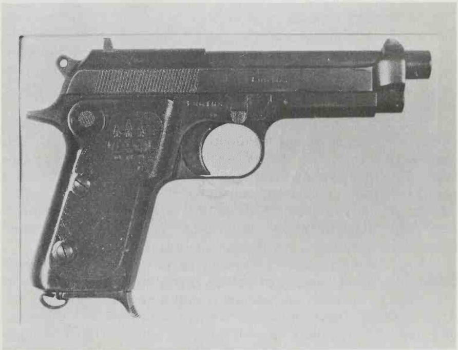
The Egyptian contract version of the Model 951. Note the differences from the standard pistol. (A. J. R. Cormack)
