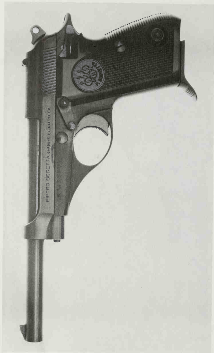
The Model 75 pistol in late form. Note the non-screw-type magazine catch button. (Beretta Archives)
