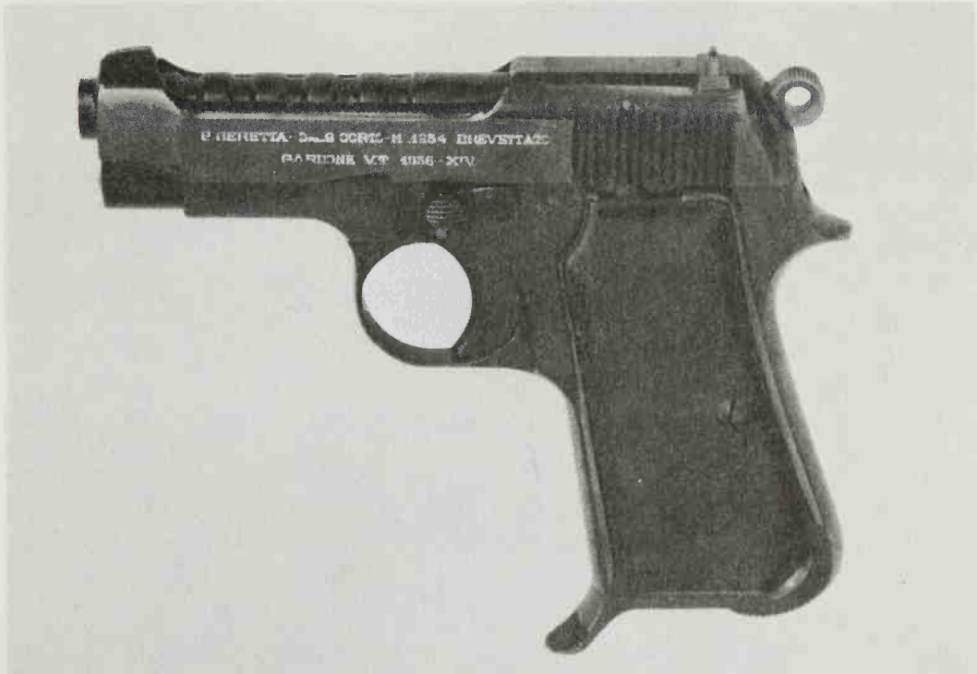
An experimental attempt at lightening the pistol by cutting wide annular grooves in the barrel. This was called the Tipo Alleggerita by the factory, and was never produced in any large quantity. (Beretta Archives)
