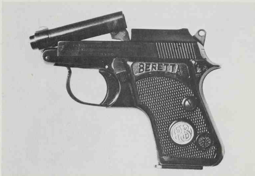
An early production Model 950, shown with the barrel open. Note the square front edges of the slide. (Beretta Archives)
