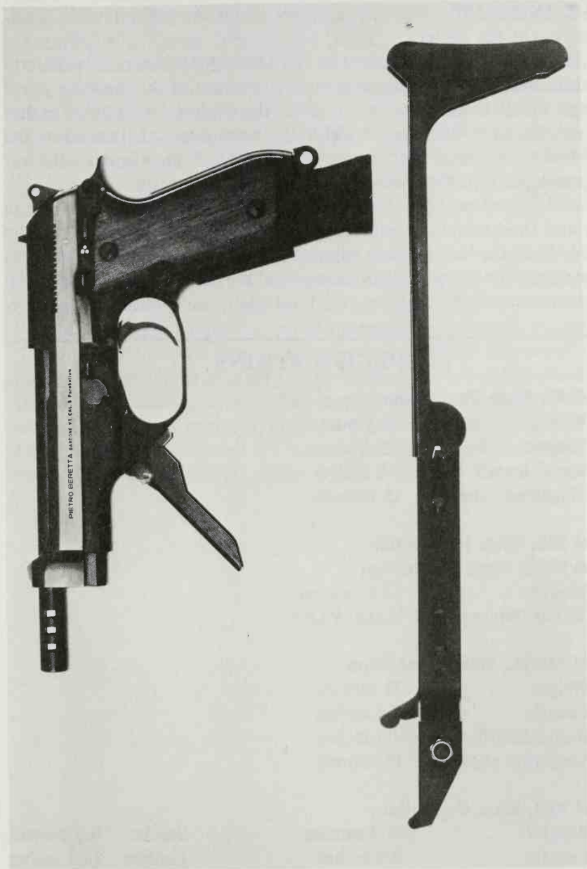
The Model 93R pistol, Second Series, shown with the shoulder stock detached. The fire selector is shown here in position for three-round bursts, and the forward handgrip is lowered.
