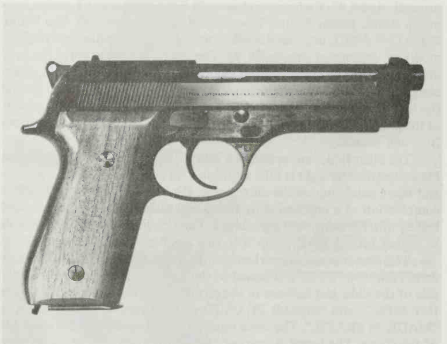
A later Model 92, with walnut grip panels. Note the flat slide, with no side steps.
