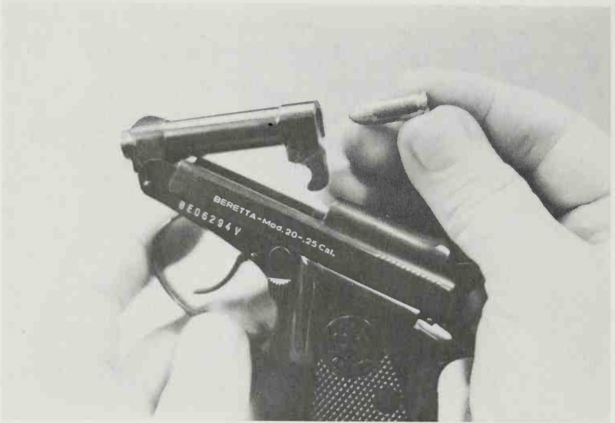
The Model 20 retained the tip-up barrel feature of the 950 Series pistols.
