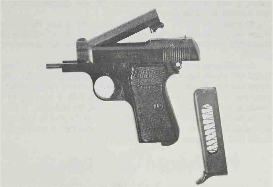
A postwar Model 1934 pistol in 9mm Corto (.380 Auto), dated 1967 on the slide. The pistol is shown partially disassembled. (Beretta Archives)
