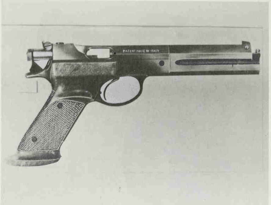
In this view, the Model 80 is shown with the bolt locked in open position. Note that the ejection port is open on both sides. (Beretta Archives)
