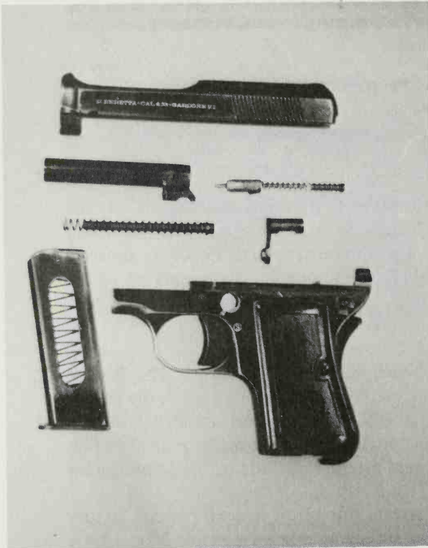
A Model 418 pistol, proof-dated 1955, serial number 98224A. Note that the steel-backed plastic grip was sometimes used, as late as 1955.
