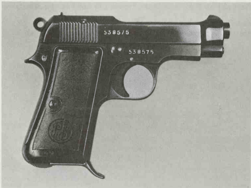
A typical Model 1935 pistol in 7.65mm chambering, from early 1944 production. It is unusual because it lacks the Fascist date in the slide marking, and bears a Swiss acceptance mark. (Author's Collection)
