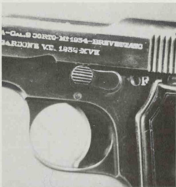
The 180-degree safety of the Model 1934 is shown in the on-safe and off-safe positions. In the former mode, the safety lever is also the takedown latch.
