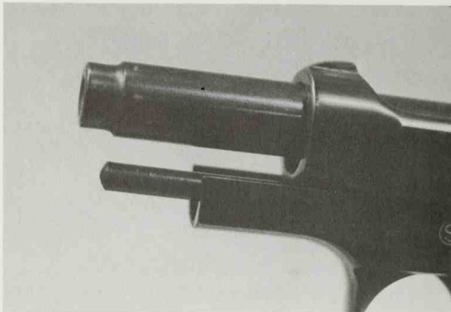
The protruding portion of the barrel at the muzzle is reduced to almost the same diameter as the later regular production barrels.
