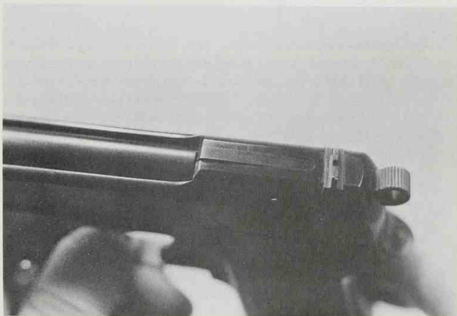
The extractor recess in the barrel of this prototype is bevelled, elevating the extractor slightly when the slide is closed.
