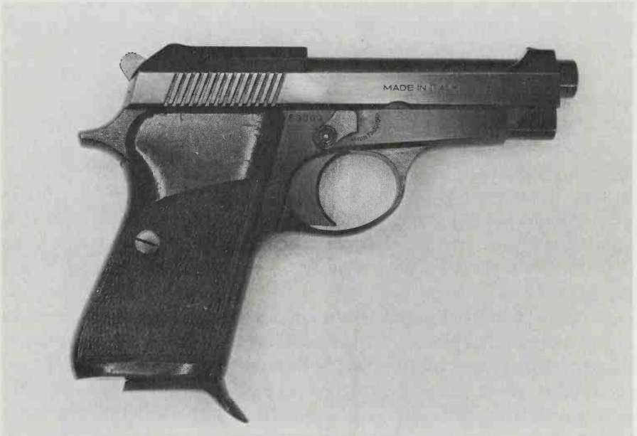
The slide markings on this pistol are "FALCON Cal. 32" and "MADE IN ITALY". The pistol bears regular Italian proof marks and a 1972 date, and the serial number is F 0003. The upper angles of the slide are flat planes, and the rear top of the slide has lengthwise grooving. This is a prototype designed for the SPESCO Corporation of Atlanta, Georgia, which had a falcon head as a trademark. The design is similar to the Model 70 pistol, and prototypes were also made in .22 caliber. This pistol was never made in regular production. (Photos courtesy of Joel Glovsky and Joseph Schroeder)
