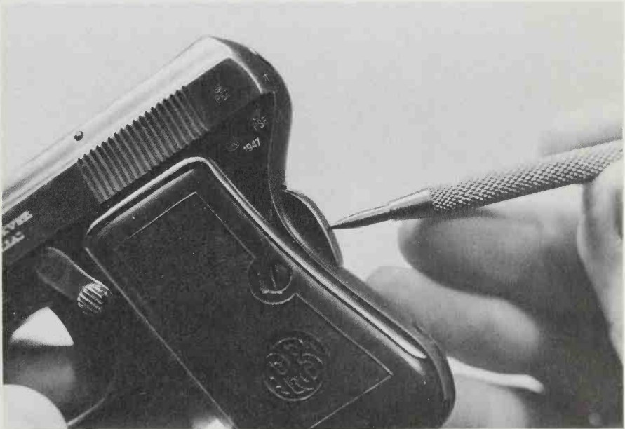
One of the last of the "hump" grip-safety pistols. Note that it is proof-dated 1947, the year in which this feature was changed.
