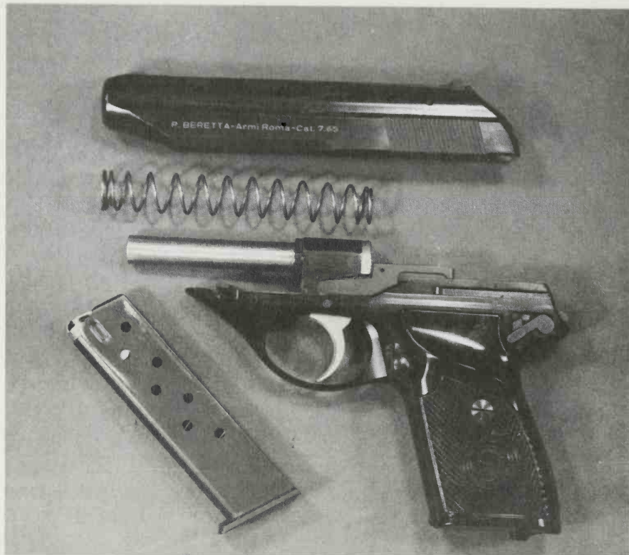
The Model 90 pistol, field-stripped. In later versions, an external slide latch was added. (Author's Collection)
