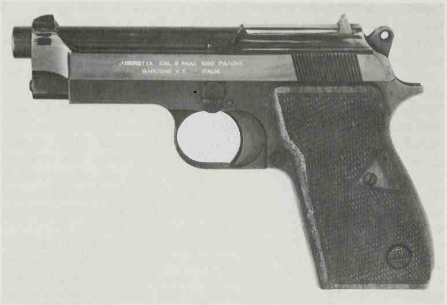
The second prototype had a Browning-style falling-barrel locking system. (Beretta Archives)
