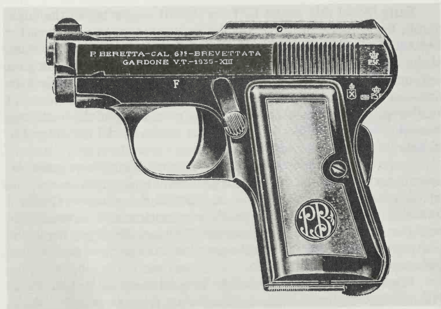
This pistol, dated 1935, is now referred to as the Model 318. It has the 1934 changes, the reshaped grip frame and the striker indicator. (Beretta Archives)
