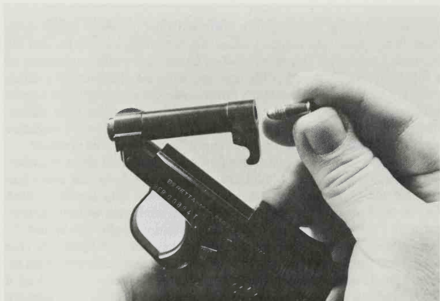
The open barrel of the 950-series pistols allows easy loading of the last round.
