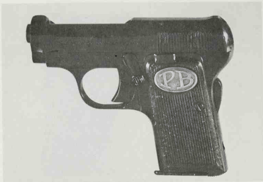
A later Model 1919 pistol. Note the formed clearance recess at the top of the grip for the disconnector arm. (Beretta Archives)
